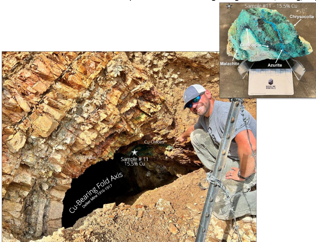
Picture 1: Photo of VP Exploration Mike Harp pointing at high-grade sample location taken at the face of the historical Delker Mine adit. Sample #11 returned 0.6m grading 15.5% Cu, 0.18 g/t Ag and 0.1% Co
