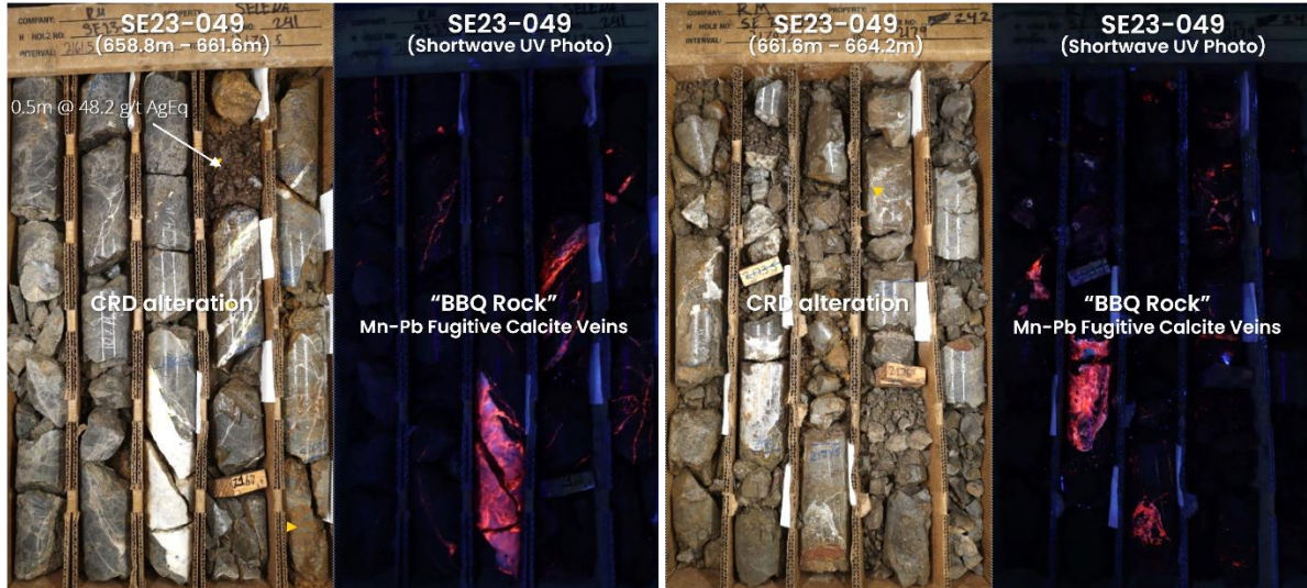
Picture 2: Shortwave UV photo of fugitive calcite veining “BBQ Rock” at depth in SE23-049. Tracking fugitive calcite veining is a proven vectoring technique in CRD systems
